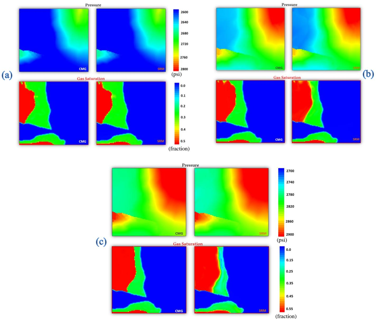
Figure 3. Pressure and Gas Saturation Distribution in the first layer of the reservoir (a) after 1 month of injection, (b) after 8 months of injection and (c) after 16 months of injection
