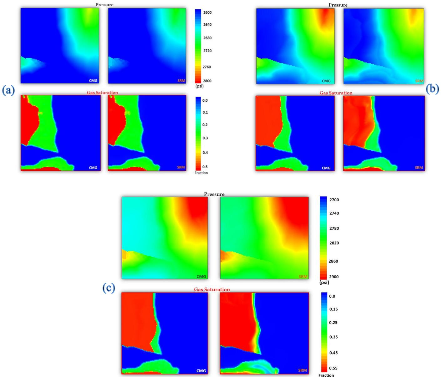
Figure 4. Pressure and Gas Saturation Distribution in the first layer of the reservoir (a) after 1 month of injection, (b) after 12 months of injection and (c) after 25 months of injection-Blind Scenario
