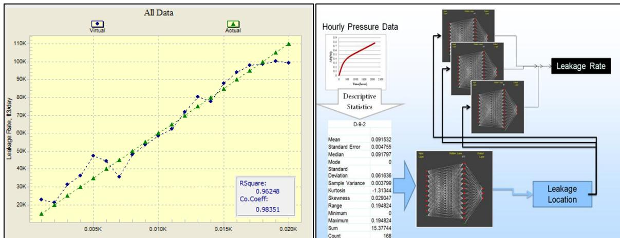
Figure 5(a). Actual leakage rate and corresponding neural network prediction (one network for each well) (b): The workflow for ILDS
