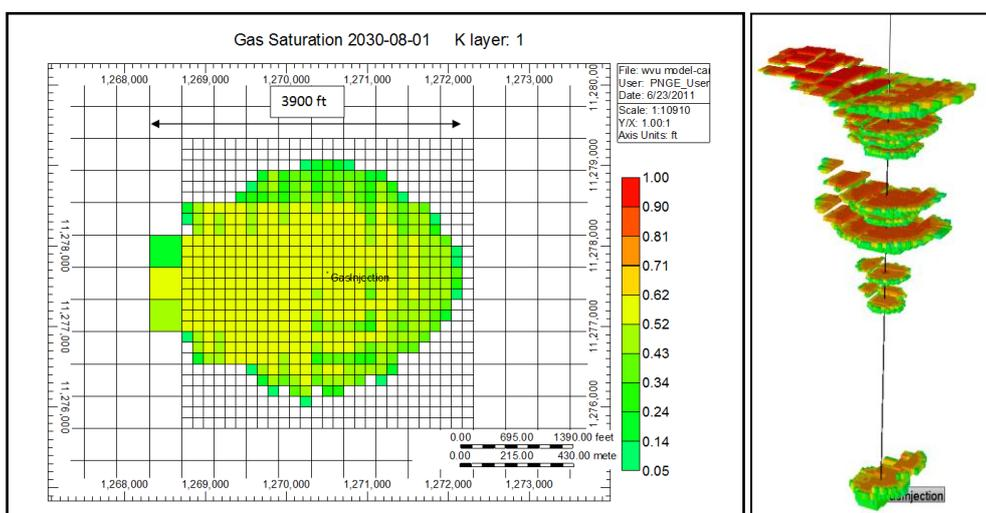
**Figure 1: Plume extension in the first layer (left) and all layers 25 years after injection**
