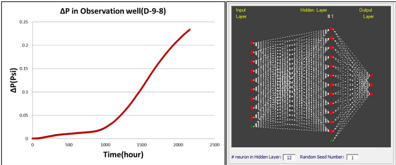
Figure 3a. Pressure change in observation well in the case that well D-9-6 leakage rate is 30Mcf/day (b): Neural Network Design for ILDS
