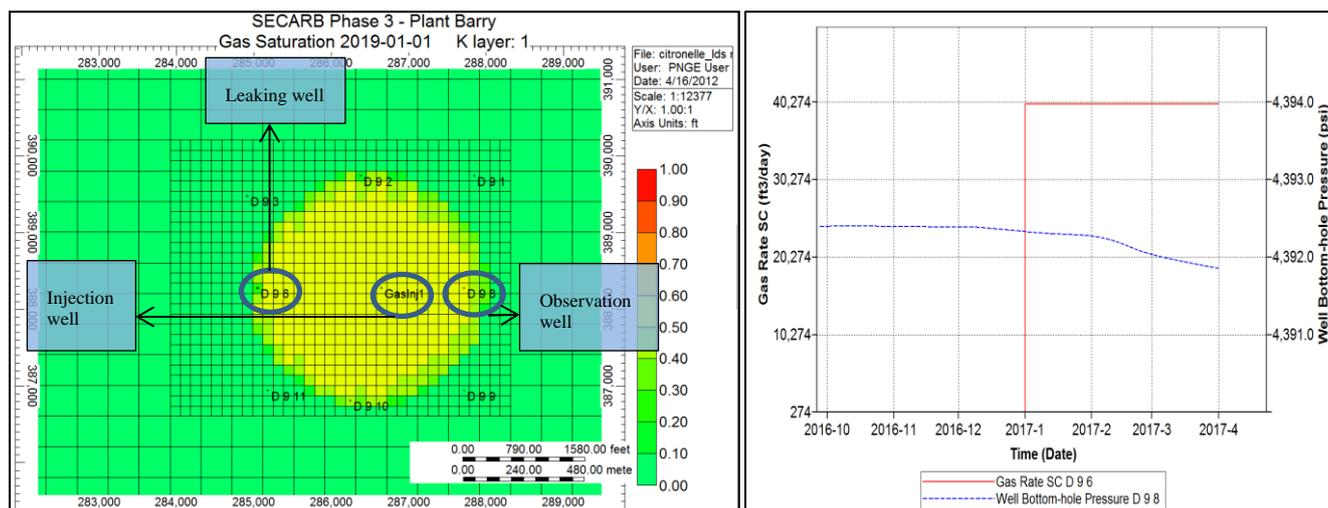
Figure 2 (a): Location of the injection and observation wells in the area of interest (b):pressure behavior in the observation well subject to the leakage rate equal to 40Mcf/day at well D-9-6
