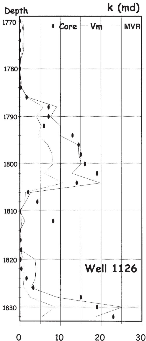
Fig. 5—Prediction models permeability vs. core measurements for Well 1126.
