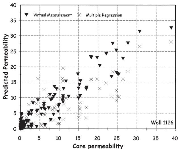
Fig. 4—Crossplot of both models performance against core measurements for Well 1126.
