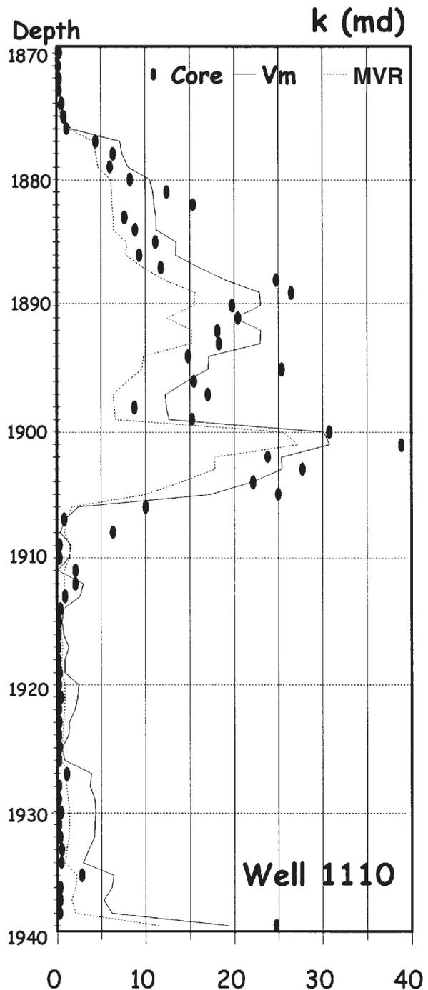
Fig. 3—Prediction models permeability vs. core measurements for Well 1110.
