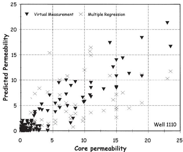
Fig. 2—Crossplot of both models performance against core measurements for Well 1110.
